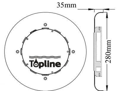
The Topline LED is designed to fit flush to the pool wall without the need for a niche. The surface mount bezel is available in stainless steel or white plastic.
